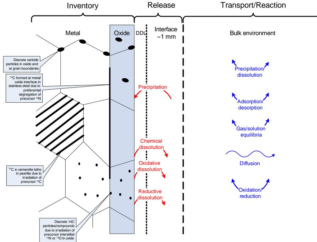
**Figure 1: Overview of Processes and Features of Possible Importance in the Development of a Source-term Model for the Release of  $^{14}\text{C}$  from Irradiated Metals.**
